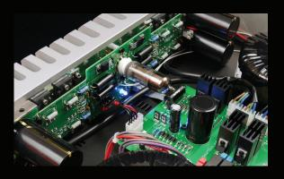
mains in conventional supplies are avoided. The addition of a choke allows a much more linear current draw instead, keeping dynamic noise under drive much lower. Premium reservoir capacitors and soft recovery diodes complete the power supply.
