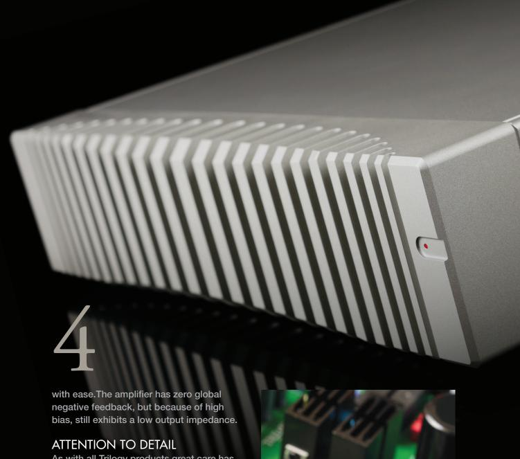
As with all Trilogy products great care has been taken with physical construction. The custom heat sink is milled from a solid billet of aluminium. The substantial mass has high thermal inertia, allowing the directly mounted output devices to operate at a constant temperature, free from the severe mechanical resonances of conventional extruded heat sinks.
