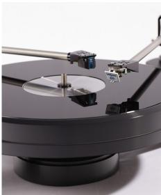
Brinkmann 'tables. The constructions materials are mostly anodized aluminum for fast transmission of harmful vibrational energy. The 22-lb. alloy/crystal-glass platter ensures speed stability and wide dynamics through the most complex musical passages.
