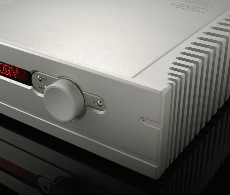
The perfectly weighted control knob and two machined stainless steel push buttons access the control menu hierarchy. All high level functions such as volume, balance and input select are quickly and intuitively accessible.
